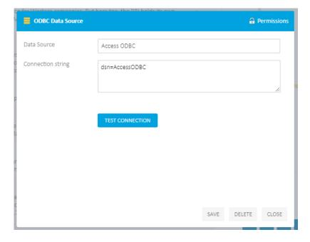
To set up an ODBC data source for MS Office applications, which are available only for 32-bit ODBC configuration, it is also required to configure Kyubit application to work in 32-bit mode. Open IIS Manager -> Application pools -> "KyubitAnalysisPool" - > Advanced Settings and set "Enable 32-bit application" to "True".
