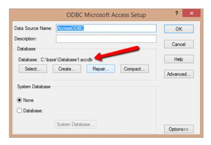
'Data Source Name' that is used for the ODBC connection on the operating system level, use to create new Data Source in Kyubit BI application.
